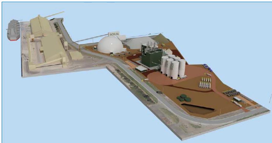
Figure 1.5: 3D model of the proposed clinker grinding facility and site layout
