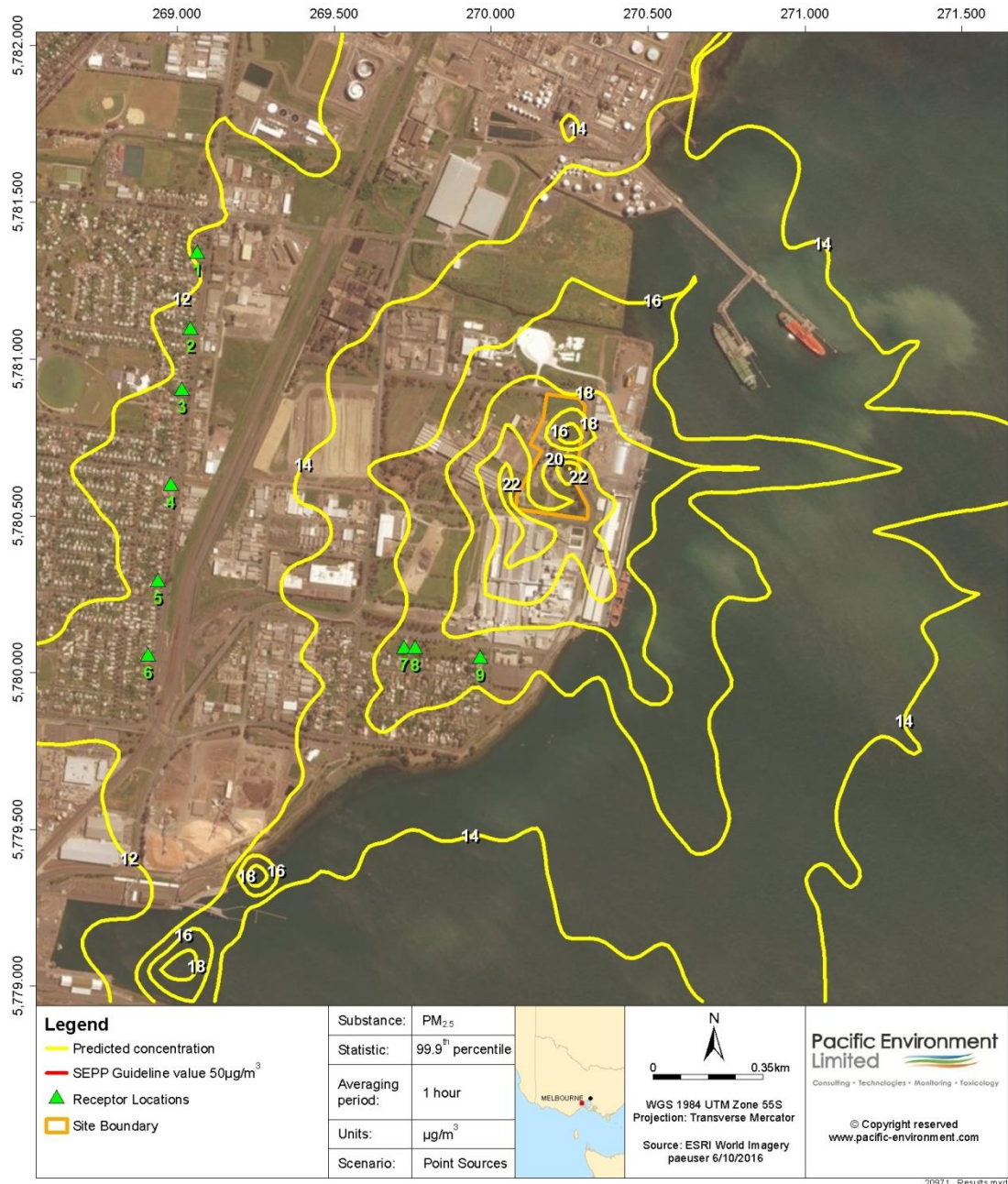
Figure 5.6: Results: PM 2.5 99.9 th percentile 1 hour concentrations from point sources only concentrations (incl background)
